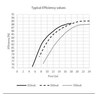
OT DX 24W G2 Typical Efficiency vs Load (230 V 50 Hz)
